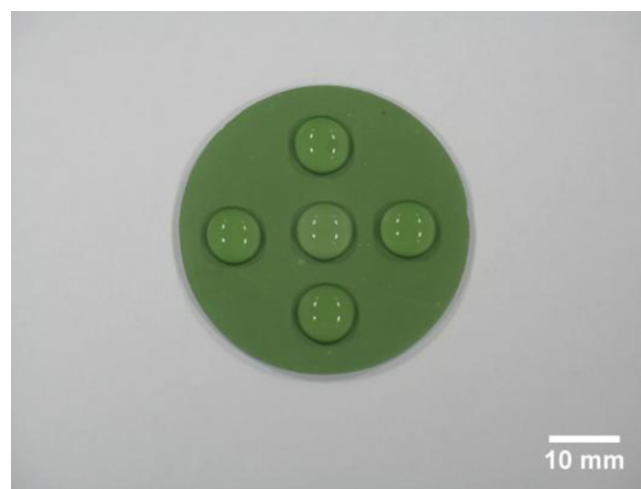
Fig. 7. Water drops deposited on sample E after a co-firing treatment at 1400^\circ\text{C} . The YSZ coating was deposited by the spin-coating technique, using a rotational rate of 3000 \text{ rpm} and a ratio Rm equal to 0.25 (sample #E). The water drops were not drained after 5 min.
